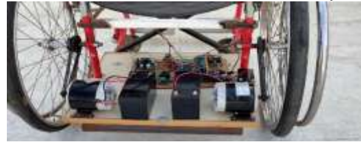
Figure 3- Wooden Base for Components
